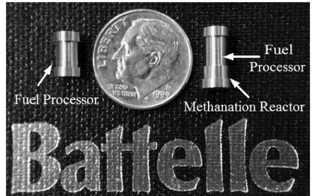
Fig. 2. Second generation micro-scale fuel processor with CO removal reactor (right) with the high efficiency reactor (left) for comparison.
