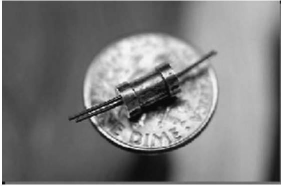
Fig. 1. Second generation micro-scale fuel processor—high efficiency.
